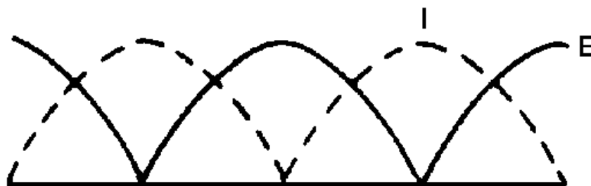
Figure 3-28.—Conventional picture of standing waves.
