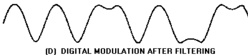
Figure 2-26D.—Simulated phase-shift keying. DIGITAL MODULATION AFTER FILTERING.
