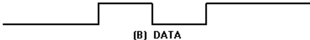
Figure 2-26B.—Simulated phase-shift keying. DATA.
